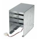
Installing up to eight (8) hard drives into your chassis is simple using one or two optional Drive Cages (PN: RDRIVECAGE), available from MAGMA. Each cage can hold up to four (4) 3.5" hard drives. The cages mount into the hard drive area in the chassis identified by a 6 in the previous graphic. If you want to install a hard drive in your system, a PCI hard drive controller card must also be installed into one of the available PCI slots.
